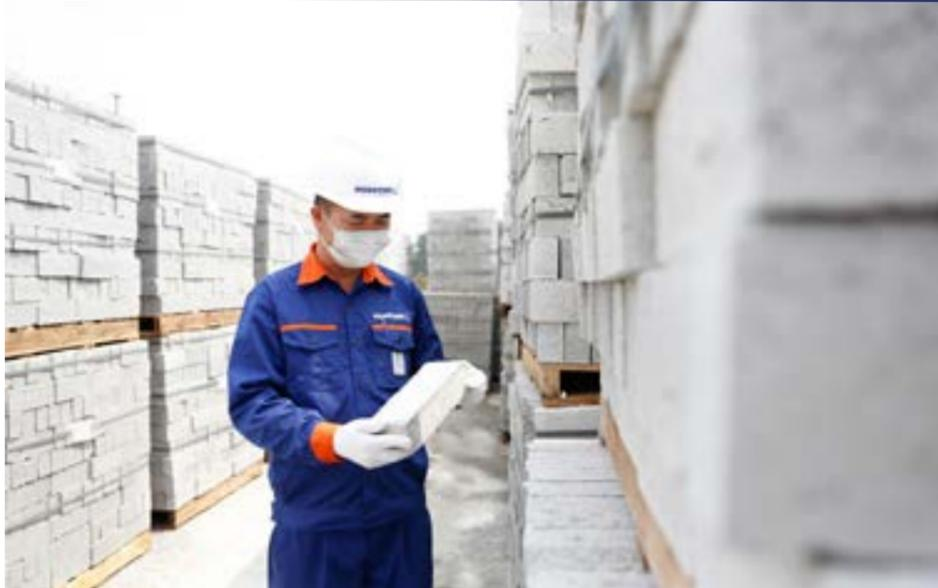
An engineer checks the quality of unburnt bricks produced from waste stone powder using Geopolymer technology
